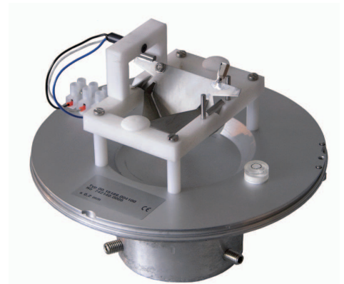
Tipping bucket mechanism
